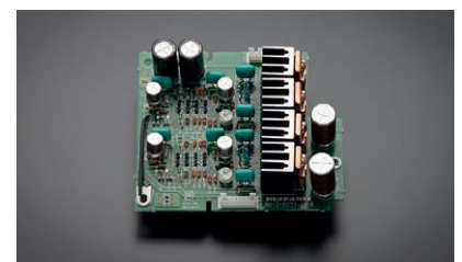
Fully discrete headphone amplifier
